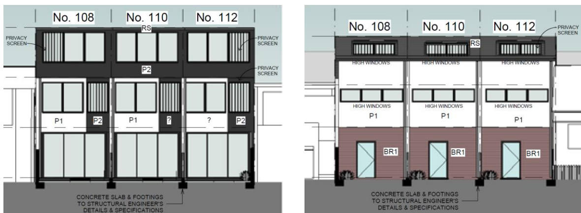
Figure 19: Proposed rear (west) elevation of the main dwellings (left) and the internal (east) elevation of the laneway structures
